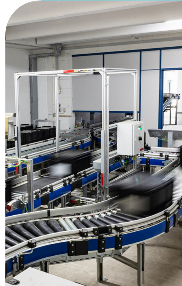
Fully automated conveyor technology for storage and retrieval.
